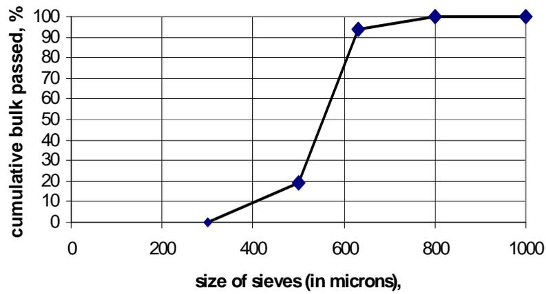
Figure 4: Particle size distribution of SiC.
