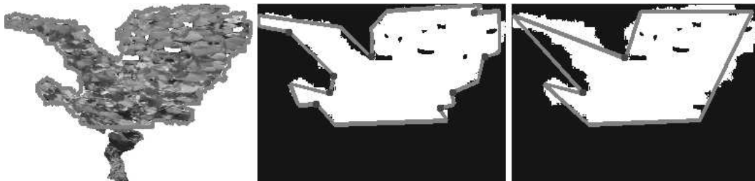
Figure 2.9: On the left, the foliage and its boundary \Omega . In the middle, and right, the DCE curve with respectively 14 and 8 vertices. Vertices of inward angle \leq \pi are shown in blue: they most likely indicate the limit between two branches regions.
