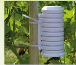
Figure 1 : solar radiation shield housing temperature logger
