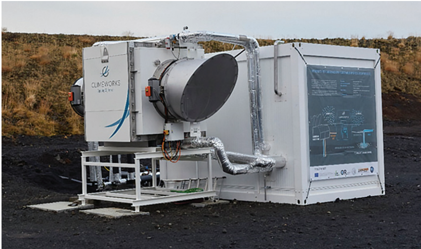
Figure 4.41 The pilot Direct Air Capture (DAC) unit at Hellisheiði was launched in October 2017. This single unit had the capacity to capture 50 t CO 2 yr -1 .
