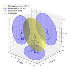
Fig. 6. Trajectory of the system within  $\mathcal{E}(P, x_*)$  and with respect to its projections
