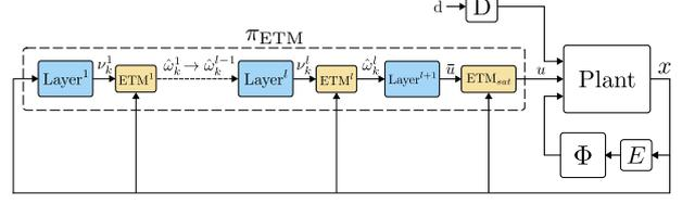
Fig. 2. Feedback system subject to ETM in the controller
