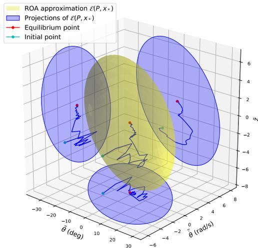
Fig. 6. Trajectory of the system within  $\mathcal{E}(P, x_*)$  and with respect to its projections
