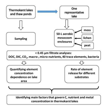
Figure 1 B: The work flow chart of the field observations, mesocosm experiments and analyses performed in this study.
