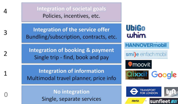
Figure 2.2: MaaS topology with different levels of integration as defined in [7]
