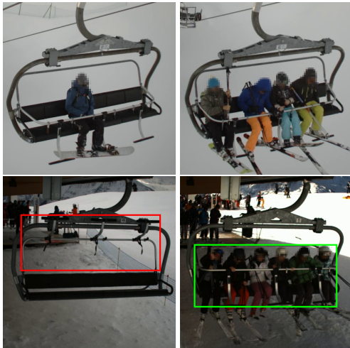
FIGURE 5 – Example images from our chairlift dataset. The two left images are from chairlift 1 and the two right images are from chairlift 2. The box annotations (open :red and close :green) are provided for the two right images, for illustration.
