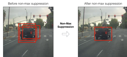
FIGURE 4 – Principe de Non-Maximum Suppression
