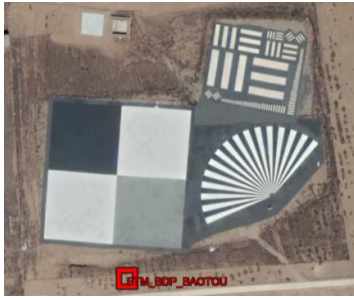
Fig. 3 Ground pattern examples (Baoutou). These patterns are currently used for MTF estimation. There are a few around the earth.
