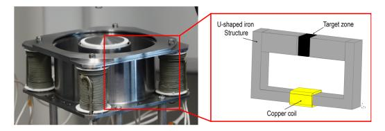
**Figure 1.** (left) A Hall-effect thruster whose shape must be optimized to obtain a target magnetic field  $\mathbf{B}_0$  inside the cavity. (**right**) A cross-section of this device is approximated into the following "toy" problem: a U-shaped iron structure is obtained (the coil was moved down from one side of the thruster to the center of the structure) with a cubic target zone in which the field must be controlled.
