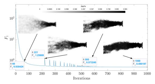
**Figure 5.** Evolution of the objective function  $F_1$  during the optimization process described in Section 4.2 to solve problem ( $P_1$ ). The small peaks correspond to the increase in the penalty parameter *n*.
