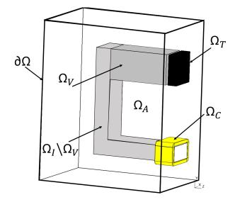
**Figure 2.** Half of the magnetic circuit studied in this article (the other half is obtained by symmetry), and the different domains that make it up: the iron domain  $\Omega_I$ , the coil  $\Omega_C$ , the air  $\Omega_A$ , the target area  $\Omega_T$ , and the variable region  $\Omega_V$ , in which we will optimize the structure.
