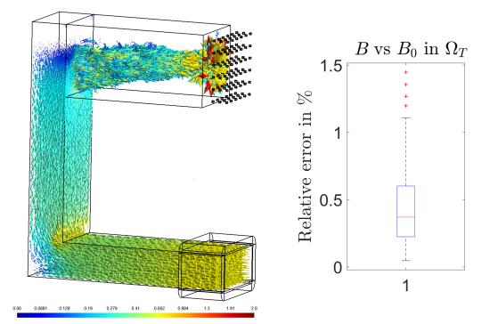
Figure 6. (left) Magnetic field inside the simulation domain for  $\rho_0^*$ . (right) Boxplot of the relative error  $\|\mathbf{B}(\rho_0^*) - \mathbf{B}_0\| / \|\mathbf{B}_0\|$  between these two fields inside the 216 cubes which discretize  $\Omega_T$  (as explained in Section 4.1).
