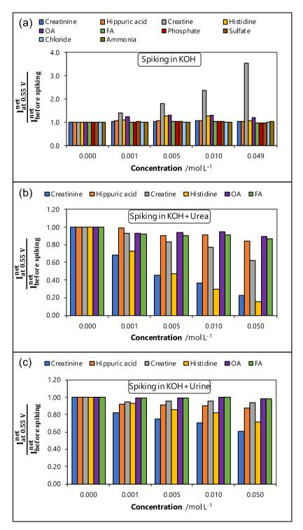
Fig. 4. Variation of the ratio of the net current of the Ni(II) oxidation signal for each spike to the net current before spiking as a function of the concentration of the spiked compound: (a) KOH, (b) urea/KOH and (c) urine/KOH media. The net currents are measured at 0.55 V.
