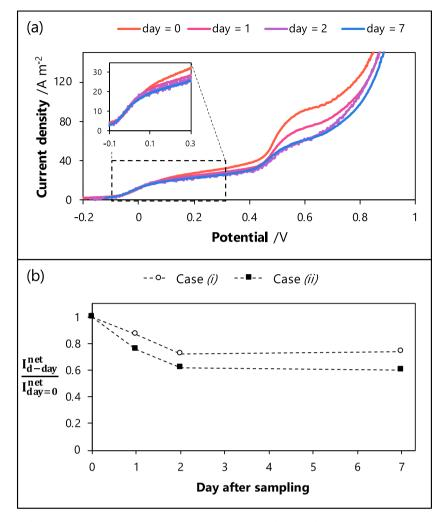
**Fig. 3.** Investigations of urine samples stability: (a) linear voltammetry of a urine solution at different days (up to 7 days) after excretion (alkalinized day-after-day, KOH 1 mol  $L^{-1}$ , 1000 RPM; 10 mV s<sup>-1</sup>; case (ii)) and (b) temporal variation of the ratio of the net current at D-day to the initial net current (observed at 0.55 V vs. Hg/HgO/OH<sup>-</sup>) obtained from the urine solution alkalinized initially (case (ii)) or day-after-day (case (ii)).
