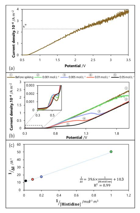
**Fig. 5.** Linear voltammograms obtained (a) with an alkalinized solution ([KOH]=1 mol L<sup>-1</sup>) and (b) when doping this alkalinized solution with histidine for concentrations varying between 0.001 and 0.05 mol L<sup>-1</sup>. (c) Determination of the affinity adsorption of histidine on nickel sites. All these results were obtained using the nickel RDE  $(3.14 \times 10^{-6} \text{ m}^2)$  at 6000 RPM and at a scan rate of 10 mV s<sup>-1</sup>.
