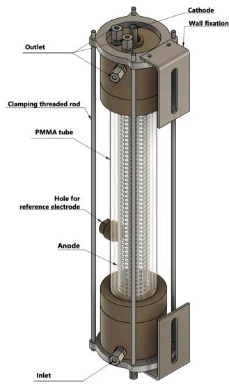
Fig. 1. Computer-aided design of pilot-scale EC reactor.
