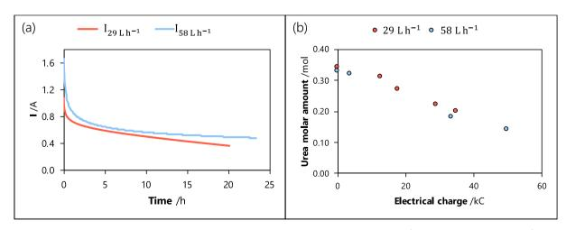
**Fig. 9.** Pilot-scale potentiostatic electrolyzes (at 0.55 V vs. Hg/HgO/OH<sup>-</sup>) of a urea synthetic solution (0.33 mol L<sup>-1</sup>) in alkaline medium (1 mol L<sup>-1</sup> KOH; 1101 cm<sup>2</sup>; undivided electrolyzer; 1 L) for two different flow rates (29 and 58 L h<sup>-1</sup>, corresponding to Re = 155 and 311): profiles of (a) the current and (b) the urea molar amount.
