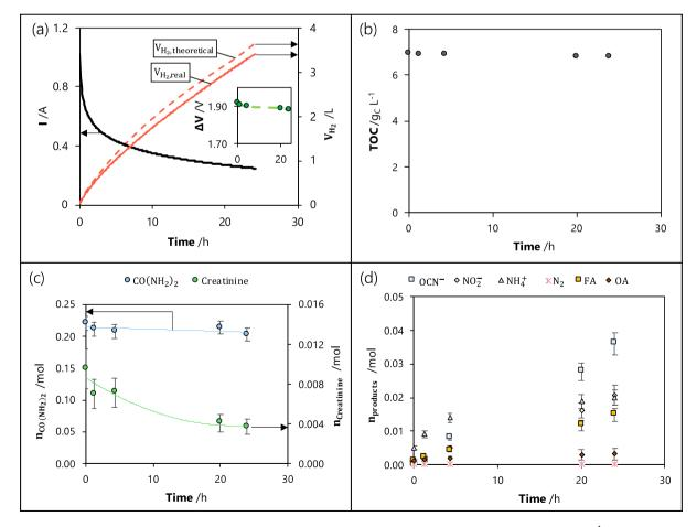
**Fig. 11.** Pilot-scale potentiostatic electrolysis (0.55 V vs. Hg/HgO/OH<sup>-</sup>) of a human urine solution (urea concentration of 0.22 mol L<sup>-1</sup>) in alkaline medium (1 mol L<sup>-1</sup> KOH, 1101 cm<sup>2</sup>, 58 L h<sup>-1</sup>, undivided electrolyzer, 1 L): temporal profiles of (a) the current and the formed  $H_2$  amount (inset: cell voltage), (b) TOC, (c) urea and creatinine molar amount, (d) molar amount of identified generated products.
