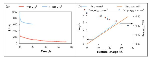
**Fig. 8.** Pilot-scale potentiostatic electrolyzes (at 0.55 V vs. Hg/HgO/OH<sup>-</sup>) of a urea synthetic solution (0.33 mol L<sup>-1</sup>) in alkaline medium (1 mol L<sup>-1</sup> KOH) (29 L h<sup>-1</sup>, undivided electrolyzer, 1 L) for two anodic surface areas (734 and 1101 cm<sup>2</sup>): (a) temporal profile of the current and (b) variation of the volume of the produced  $H_2$  (continuous lines) and of the molar amount of unconverted urea (circles and squares) during electrolysis.
