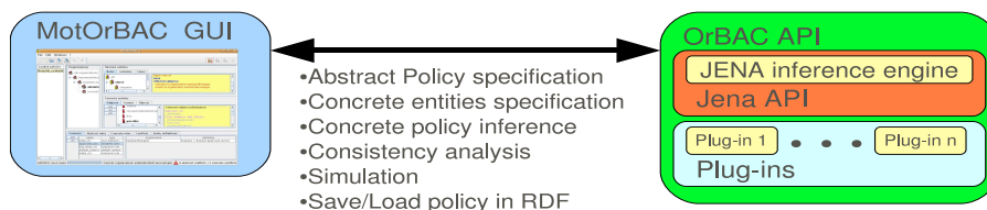
Fig. 1. The MotOrBAC tool architecture which is based on the java OrBAC API
