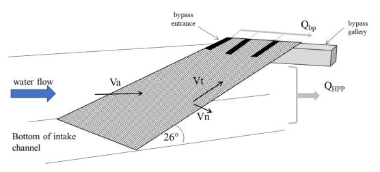
Fig. 3. Hydraulic parameters of velocity and discharge on the inclined low bar spacing rack (side view) with surface entrances to the bypass: Va – approach, Vt – tangential, Vn – normal velocities,  $Q_{HPP}$  – HPP intake discharge,  $Q_{bp}$  – bypass discharge.
