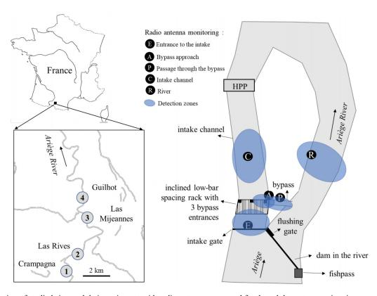
Fig. 1. Localisation of studied sites and their equipment with radio antenna array used for the eel downstream migration survey (all four sites have the same configuration and similar radio antenna array; only Crampagna could not be equipped with the antenna A; detection zones in blue).
