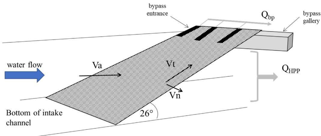
**Fig. 3.** Hydraulic parameters of velocity and discharge on the inclined low bar spacing rack (side view) with surface entrances to the bypass:  $V_a$  – approach,  $V_t$  – tangential,  $V_n$  – normal velocities,  $Q_{HPP}$  – HPP intake discharge,  $Q_{bp}$  – bypass discharge.
