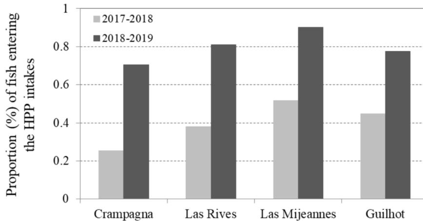
**Fig. 4.** Proportion of eels detected at the entrance of each studied HPP intake (antenna E) per study season (100% – all detected fish (including dam passages) crossing the complex with HPP turned-on).
