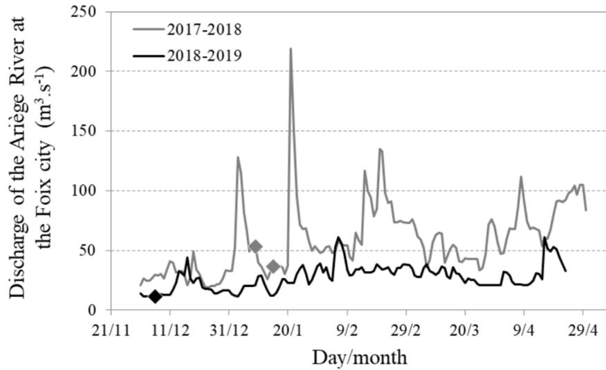
**Fig. 2.** Mean daily discharge of the Ariège River at Foix (about 10 km upstream of the study area) during the study period (dots: days of eel releases, discharge data source <http://hydro.eaufrance.fr>).
