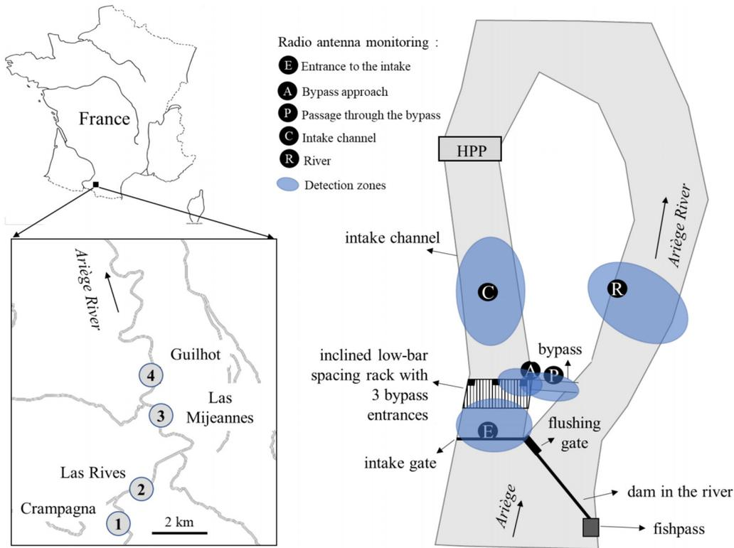
**Fig. 1.** Localisation of studied sites and their equipment with radio antenna array used for the eel downstream migration survey (all four sites have the same configuration and similar radio antenna array; only Crampagna could not be equipped with the antenna A; detection zones in blue).
