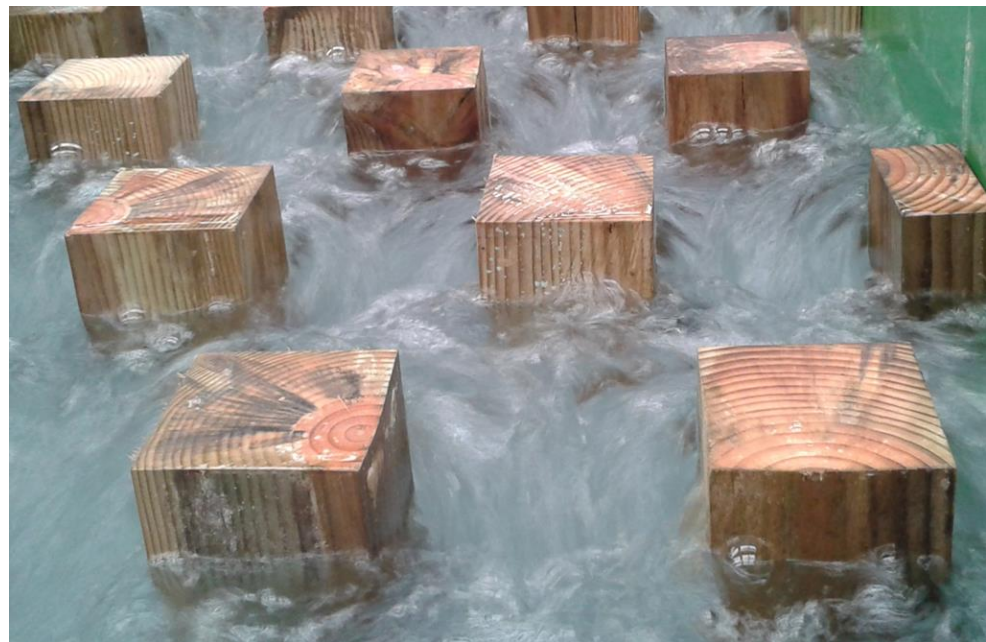
Figure 1. Picture of the flume in operation.
