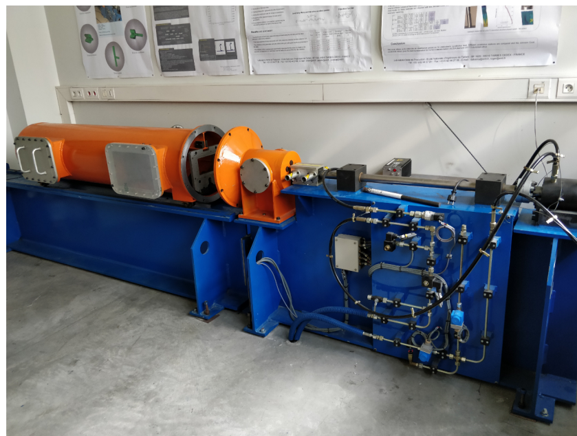
Figure 2. The Taylor gas gun device in LGP.
