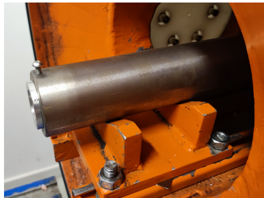
Figure 3. The target and the massive target support on the double V.
