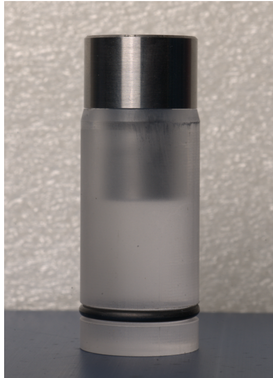
Figure 5. Projectile for the dynamic tensile test.
