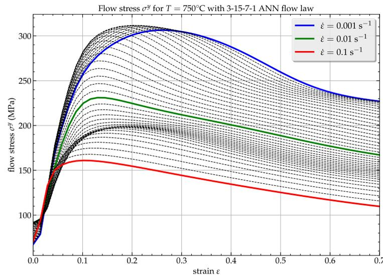
**Figure 12.** Predicted flow stress  $\sigma^y$  as a function of  $(\epsilon^p, \dot{\epsilon})$  for a fixed temperature  $T = 750 \text{ }^\circ\text{C}$  using the 3-15-7-1 model.
