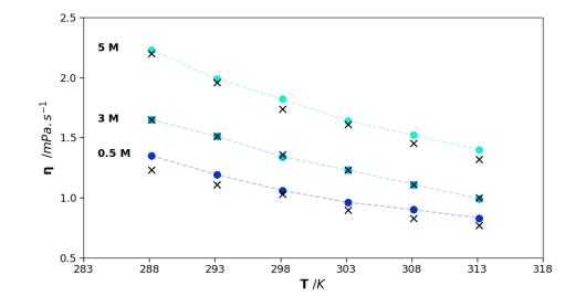
Fig. A.2 Effect of the presence of 0.33 mol.L<sup>-1</sup> urea on the viscosity of alkaline solutions with different concentrations of potassium hydroxide. The crosses correspond to the viscosities of the alkaline solutions when adding urea at 0.33 mol.L<sup>-1</sup>.
