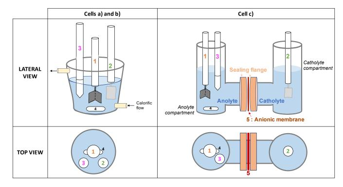
Fig. 1. Experimental setup used for a) i-E curves b) undivided cell for preparative electrolysis c) un/divided cell for preparative electrolysis. Working electrode (WE) and counter electrode (CE) are identified as 1 and 2. Reference electrode is labelled 3. In the case of electrolysis, a magnetically stirring bar (mark 4) was used to mix the electrolyte solution. In case of divided cell, the membrane separator (mark 5) holds in place by flanges that maintain the seal.
