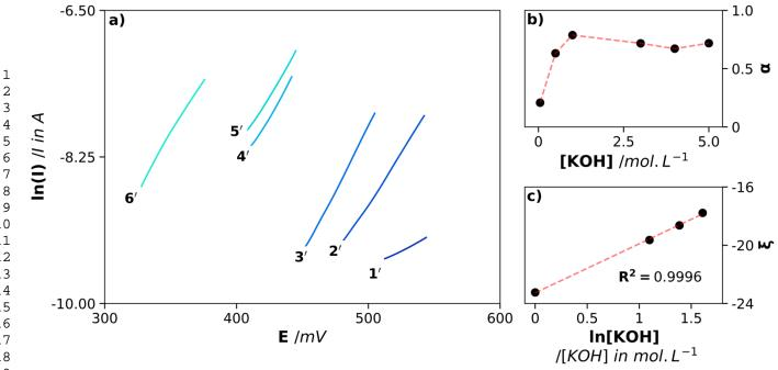
Fig. 8. a) Butler-Volmer analysis of voltammogram 1' to 6' extracted from Fig. 7-b. Figure b) shows the dependency of the anodic charge transfer coefficient  $\alpha$  against the hydroxide concentration. Figure c) highlights the intercept of Butler-Volmer analysis against the natural logarithm of KOH concentration.
