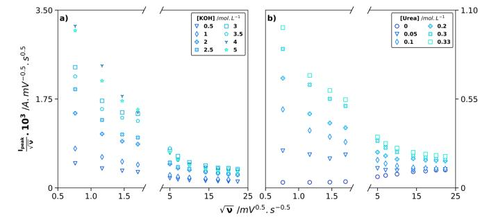
Fig. 5. Evolutions of the ratio between the current magnitude of anodic peak and  $\sqrt{\nu}$  at different concentrations of a) KOH in a solution of 0.33 mol.L<sup>-1</sup> urea and b) urea in a solution of 1 mol.L<sup>-1</sup> KOH. Results extracted from the current potential curves (not shown here) were plotted for various concentrations of a) KOH from 0.5 to 3 mol.L<sup>-1</sup> or b) urea from 0 to 0.33 mol.L<sup>-1</sup>.
