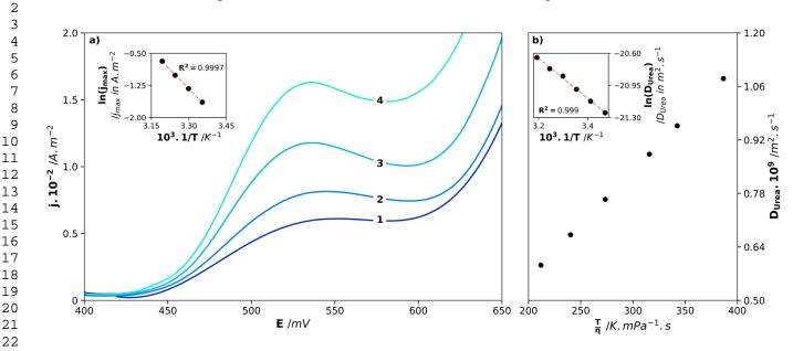
Fig. 9. a) Effect of temperature on the voltammograms obtained at 0.66 mV.s<sup>-1</sup>, on nickel RDE in a 1 mol.L<sup>-1</sup> KOH solution containing 0.33 mol.L<sup>-1</sup> <sup>1</sup> urea. The temperature used was 298 K (1), 303 K (2), 308 K (3) and 313 K (4).  $\omega = 200$  RPM. Inset:  $ln(j_{max}) = f(1/T)$  plotted to determine the activation energy of the global process.
