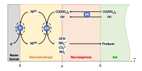
14 Fig. 3. Schematic representation of the indirect oxidation of the urea, by the electromediation of the system Ni(OH)<sub>2</sub>/NiOOH operating on the 15 surface of a massive nickel anode, and in presence of alkaline medium. ER, HCR, and D/M indicate respectively the locations where the NiOOH 16 electrogeneration reaction, the heterogeneous catalytic reaction and the mass transport (limited by the diffusion) take place.
