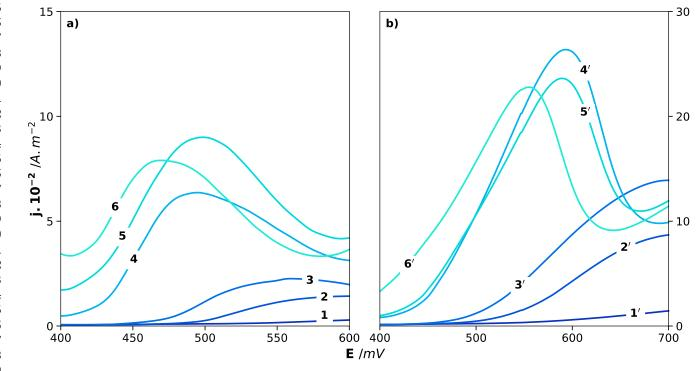
Fig. 7. Effect of KOH concentration by linear voltammogram of nickel RDE in a solution containing 0.33 mol.L<sup>-1</sup> urea at a) 1.36 and b) 500 mV.s<sup>-1</sup> without agitation at 298 K. The potassium hydroxide concentration used was 0.05 mol.L<sup>-1</sup> (1-1'), 0.5 mol.L<sup>-1</sup> (2-2'), 1 mol.L<sup>-1</sup> (3-3'), 3 mol.L<sup>-1</sup> (4-4'), 4 mol.L<sup>-1</sup> (5-5') and 5 mol.L<sup>-1</sup> (6-6').
