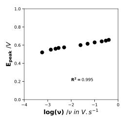
Fig. E.1 Evolution of the anodic peak potential against the logarithm of the potential scan rate
