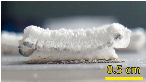
Fig. 14. Lateral perspective of a cuboid of 1.4 \times 1.4 \times 0.4 cm displaying mushroom-like deformation caused by overheating the upper surrounding regions of the part.
