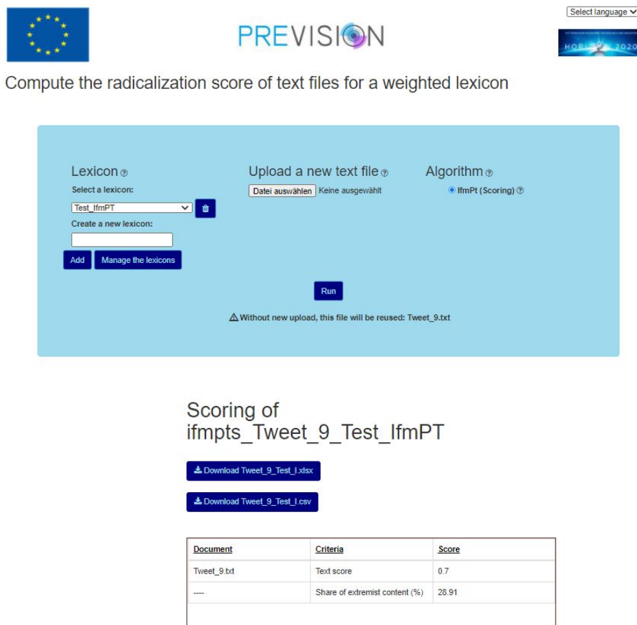
Figure 6. This figure shows the API of the application that calculates the radicalisation score of text files for a weighted lexicon. First, the user selects the lexicon to be used and the file or directory to analyse (top part of the figure). As a result, the overall score of the texts is displayed.
