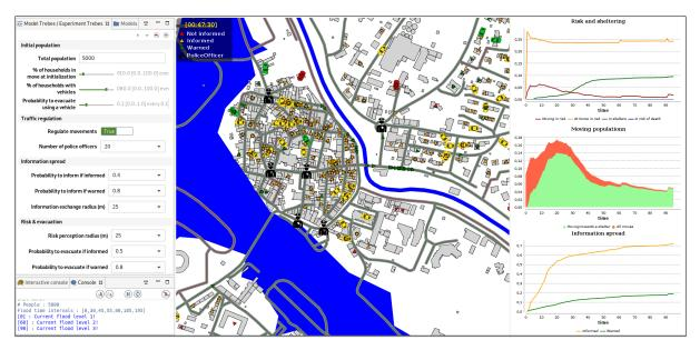
Figure 7. The graphical interface of the self-sheltering simulator under the GAMA platform with input parameters (top-left), real-time outputs and charts (right), and the map of the study area with the simulated agents (vehicles, pedestrians, police officers)
