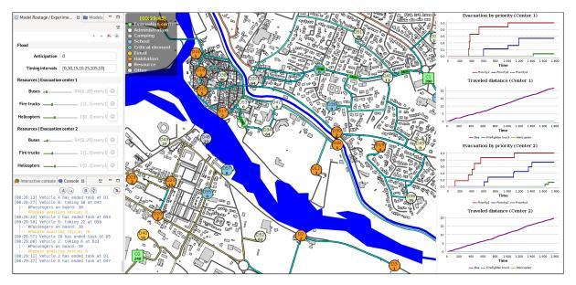
Figure 8. The graphical interface of the evacuation simulator under the GAMA platform with input parameters (top-left), log of evacuation activities (bottom-left), real-time outputs and charts (right), and the map of the study area with the simulated agents (emergency vehicles, rescue demands)
