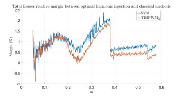
Fig. 5. Relative margin, ( $\epsilon_r$  eq.(21)) for optimal harmonic injection compared with SVM and THIPWM  $\frac{1}{6}$  applied to Total losses ( $\mathcal{P}_{tot}$  eq.(7)) for N = 5
