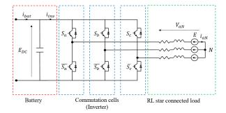
Fig. 1. Scheme of the RLE model
