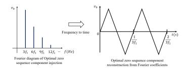
Fig. 2. Principle of ZSCM, a zero sequence component is generated from the computed optimal Fourier specter (here is represented as an example the SVM one).
