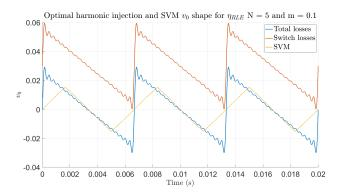
Fig. 8. Normalised and centred  $v_0$  comparison between harmonic injection and SVM for Total losses (eq.(7)) and considering switches losses (eq.(12)) for N=5 and m=0.1
