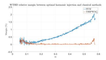
Fig. 4. Relative margin,  $(\epsilon_r$  eq.(21)) for optimal harmonic injection compared with SVM and THIPWM  $\frac{1}{6}$  applied to WTHD (eq.(2)) for N=5
