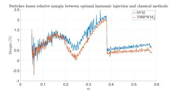
Fig. 6. Relative margin,  $(\epsilon_r \text{ eq.}(21))$  for optimal harmonic injection compared with SVM and THIPWM  $\frac{1}{6}$  applied to switches losses only  $(\mathcal{P}_K \text{ eq.}(12))$  for N = 5
