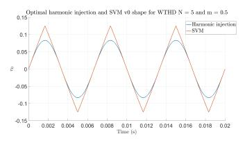
Fig. 7. Normalised and centred  $v_0$  comparison between harmonic injection and SVM for WTHD (eq.(2)) considering N=5 and m=0.5
