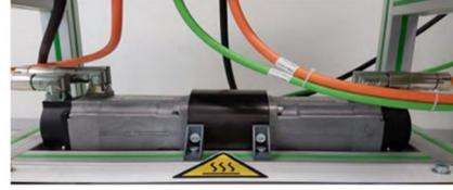
Fig. 4. The tested PMSM (left) coupled to the load motor (right)
