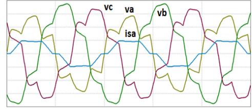
Fig.8. Perturbed voltages source and  $i_{sa}$  source current before filtering (50V-5A-5ms/div)
