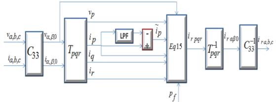
Fig.5. Bloc diagram to extract the reference currents based on the modified p-q-r theory
