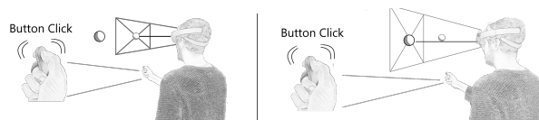
Figure 8: Setup of one trial for selection outside the FoV task with (left) the first target placed in the center of the initial FoV and the user performs a Button Click and (right) the user's head rotated 45° to the left to point at the second target and s/he performs a Button Click.
