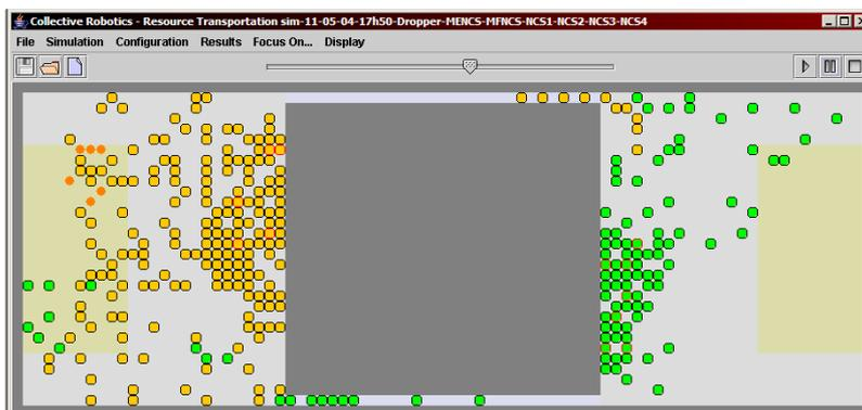
**Fig. 1.8** The environment of the resource transportation problem is composed of: a claim room (at left), a laying room (at right) and two narrow corridors (at top and bottom). Robots pick boxes against the left wall of the claim room (claim zone) and drop them against the right wall of the laying room (laying zone).
