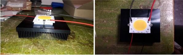
**Figure 3:** The first prototype LED + TEG1+dissipator
