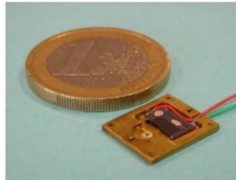
Fig. 1. Electrostatic MemS inside its packaging
