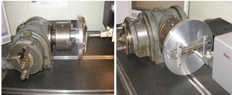
*Fig. 3 Device for roughness measurements*
